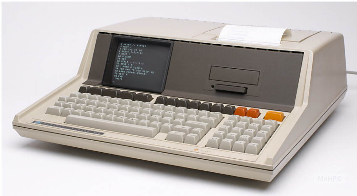
HP – 85 Note the small built in screen and the roll of thermal paper used to output data
